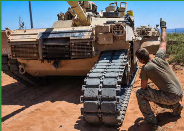
Spc. Derek Sparks, a track vehicle mechanic with 106 SPT helps repair a broken track on a M1A2 SEP V2 Abrams Tank. (Photo by Sgt. Brittany Johnson)
